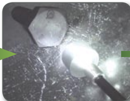
▫ Retrieval magnet deployed
