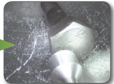
▫ Loose bolt retrieved
