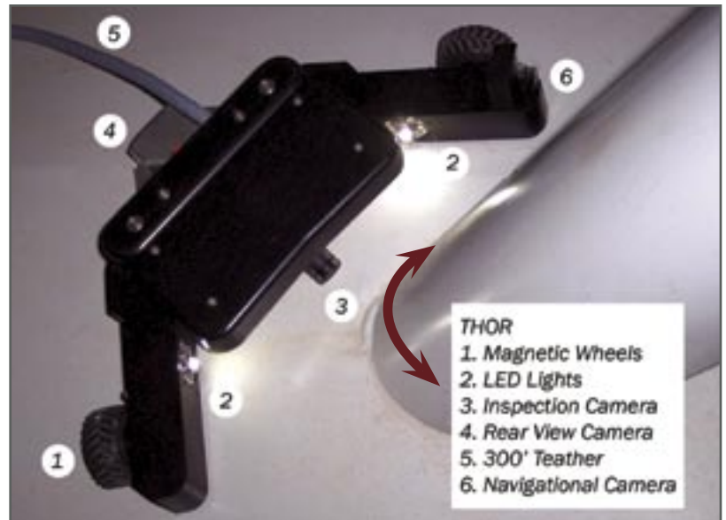
▫ CRDM inspection with THOR on mock-up
